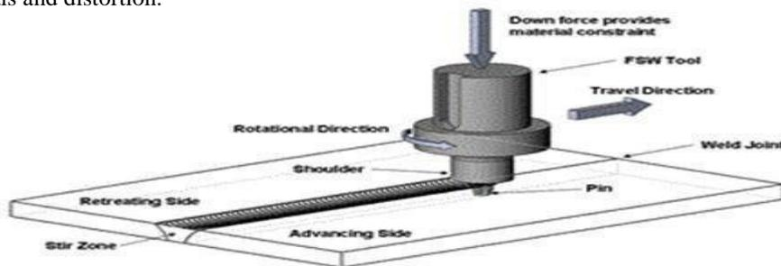
Figure 1 Schematic diagram of FSW Process
